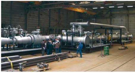
Besides quantity and quality measurement our Metering Systems are often supplied including fluid filtration, pressure regulation and flow control.
